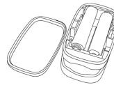
Figure 3 Installation des piles
