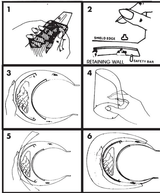
1. Peel the shield. There is a protective film on both sides of the shield.
