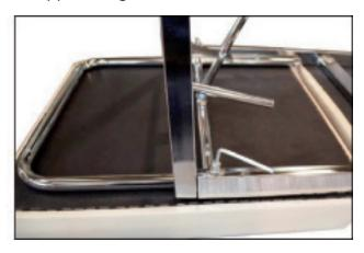
Insert the adjustment rod into its housing (the plate hole).
