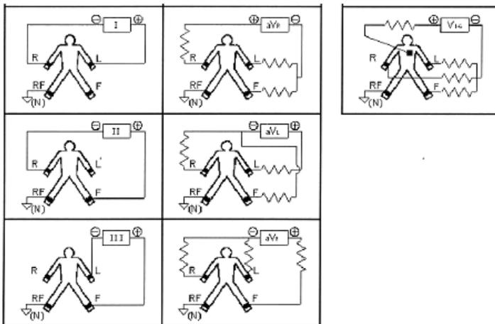
Figura 6-4 Sistema conductor
