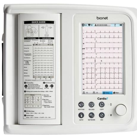
Cardio7e/Cardio7 is an electrocardiogram (ECG) device capable of measuring and recording 12 channels of cardiac signals of patients. The device enables operators to record cardiac signals, review them using various viewing modes, and perform automatic detection of cardiac conditions.
