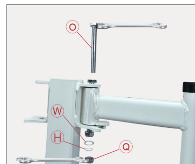
19. Insert the long screw into hole, lock with the nut.
