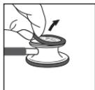
To remove the Littmann tunable diaphragm, pinch the rim of the diaphragm with your thumb and index fingernails; pull and lift the diaphragm from the chestpiece.
