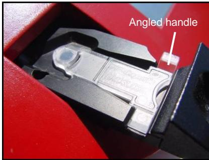
Figure 15 - Correctly positioned cuvette
