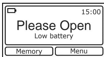
The battery symbol indicates its remaining capacity. The device displays the warning “Low battery” at low capacity. If the battery is not recharged, the device switches off after a while.
