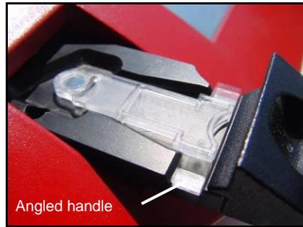
Figure 16 - Incorrectly positioned cuvette
