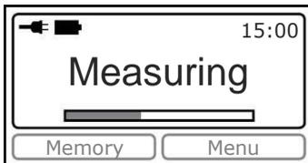
Closing the cuvette holder starts the measurement.
