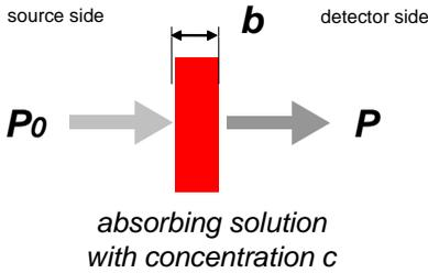
Figure 25 – Principle of photometric measurement
