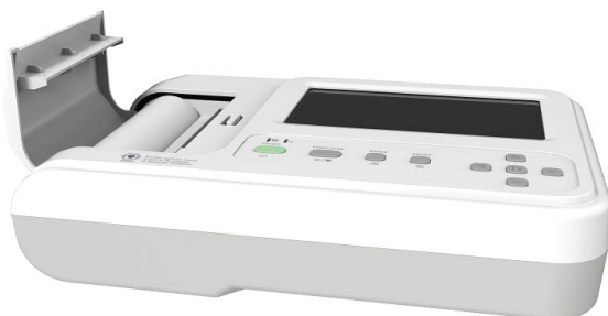
Figure 6-1 Installation of recording paper
