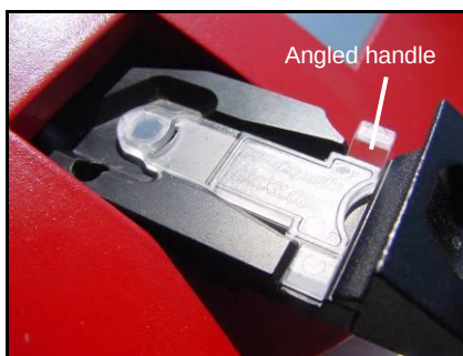
Figure 15 - Correctly positioned cuvette
