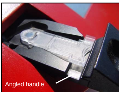
Figure 16 - Incorrectly positioned cuvette
