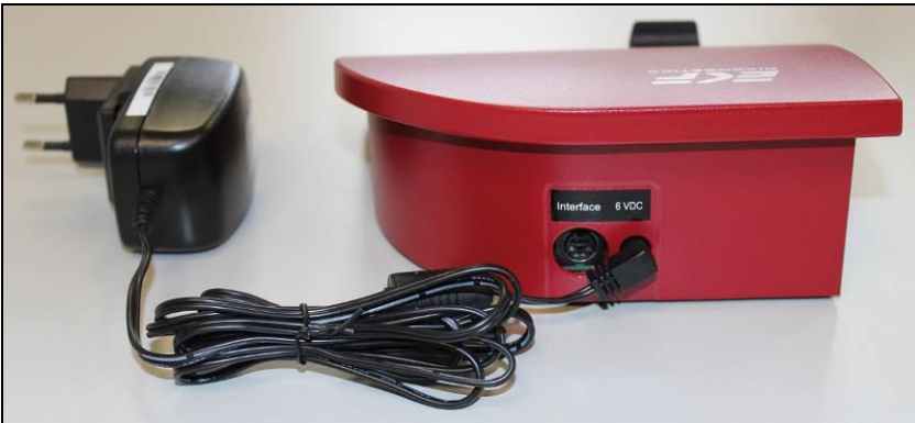
Figure 2 - Connection of mains adaptor
