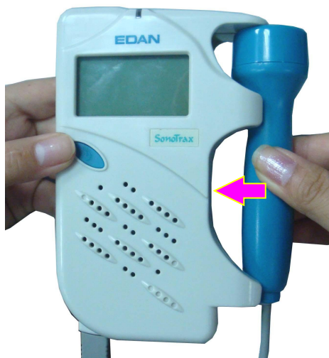
Figure 3-5 Placing the probe
