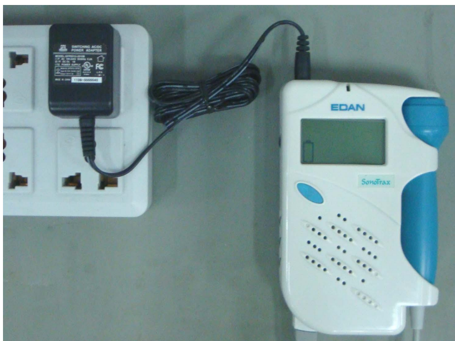
Figure 3-7 Charge du bloc-batterie Ni-MH
