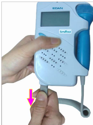
Figure 3-6 Removing the probe
