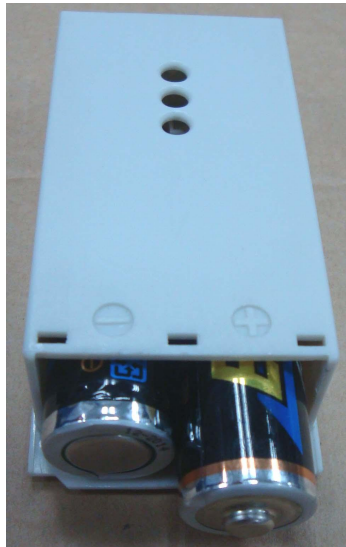
Figure 3-2 Putting batteries into the compartment cover
