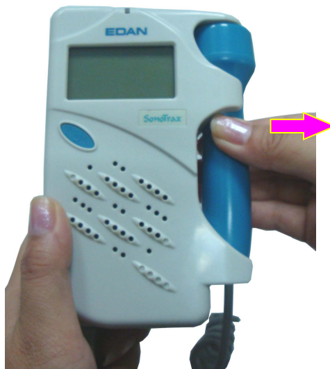
Figure 3-4 Taking out the probe
