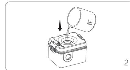
2. Fill the water tank with distilled water. please notice that do not pour the hot water into it;
