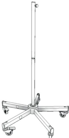
**WARNING:** Verify that the stem is tightly secured and that the mobile version is stable and parallel to the floor. Ensure that all wheels rotate freely.
