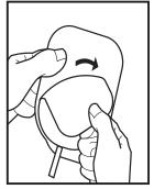
Peel off the protective cover of the conducting gel of the pads
