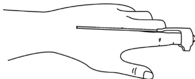
Reference diagram of SpO<sub>2</sub> probe placement
