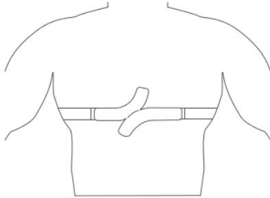
5. In order to obtain an accurate measurement, it is essential that all of QardioCore's electrodes remain in contact with your skin at all times. We have designed QardioCore to suit a multitude of body shapes and chest types, allowing for you to make slight modifications to how QardioCore is worn to maximize the recording quality and comfort on an individual level. If the ECG data is erratic or does not appear, you can try these tips:
