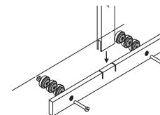
**Please note:** to avoid damaging the scale when in use, the heel stop must be supported against the wall. Therefore you must attach sufficient spacers behind the heel stop so that the last one contacts the wall.
