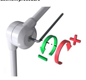
Remove the adhesive to access the joint in question. Using the Allen key, adjust the screw alongside the joint.
