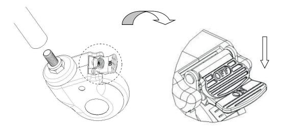
Unlock the caster: Press the OFF button with your foot and unlock the castor when you hear a "click".
