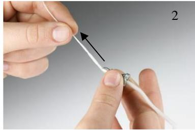
Having cleaned the channels thoroughly, the tip of the probe must be refitted. Offer the tip of the probe to the main body, being careful to align the guide pin *A* presented by the body with the hole *B* located in the tip, as illustrated in the figure below. Retighten the screw collar.
