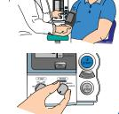
Set P-SET 3 to desired target value or to AUTO (optimum inflation pressure)
