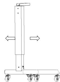
Take out the round machine hexagon socket screw M8\*25, flat washer  $\phi 8$ , spring washer  $\phi 8$  from the screw package, first install the screws on both sides of the riser, and finally install the screws on one side of the riser.
