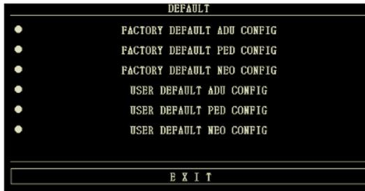
In this sub-menu, you can select both the factory default and the user-defined default. Also in this sub-menu, you can save the current system configuration as the user-defined default configuration. But at this time, the system will automatically save all the setups in the parameter menu, ECG gain and filter way as the user-defined default configuration according to the patient type. Also, a dialog box "CONFIRM TO SAVE" will pop up.
