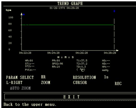
The y-axis stands for measured value and x-axis stands for time. The symbol "↓" in above figure is the cursor of trend graph. The value that the cursor points to, is displayed under the trend graph, and its corresponding time is displayed above the trend. Other trends except NIBP trend are displayed in continuous curves. In NIBP trend graph, the symbol "\*" represents the coordinate of the NIBP value.
