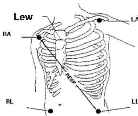
Electrodes Placement (5-lead)
