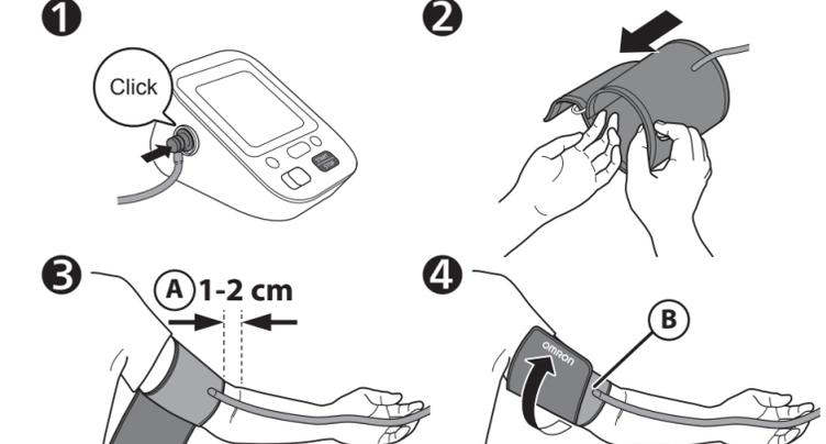
A Tube side of the cuff should be 1 - 2 cm above the inside elbow.
