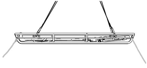
**⚠** Before lifting or lowering, after carrying out all the safety checks necessary for handling, adjust the harness and/or distribute the load inside the basket stretcher in order to balance its horizontal position when it is then handled.
