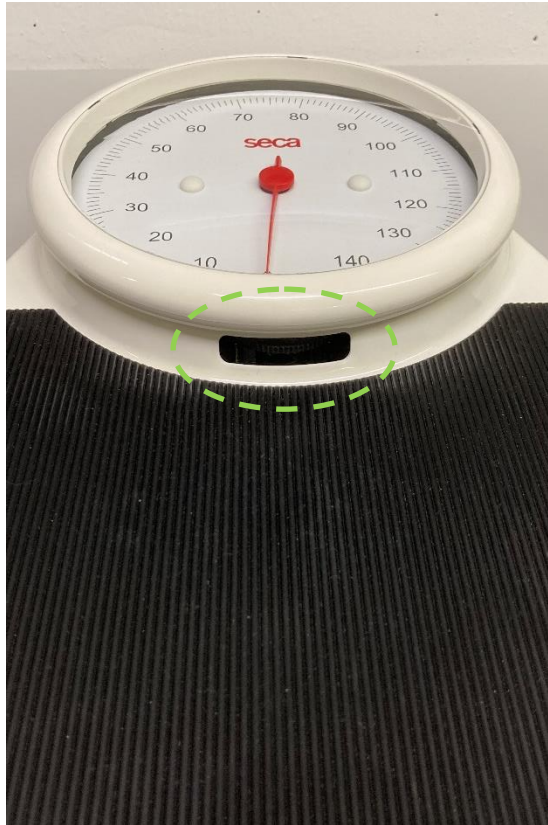
Figure 6: front view with zero setting device
