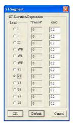
The physician can "choose lead" according to what he needs to input the parameter. The parameter should be between 0.01 and 0.3. If the input number is out of the range, the computer will display:
