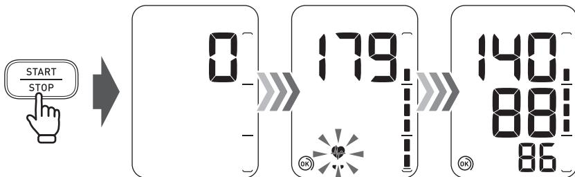
**When the START/STOP button is pressed, the measurement is taken and saved automatically.**
